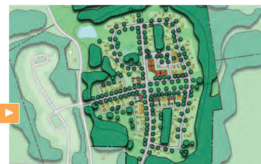
Conservation Design: Increases density of lots while decreasing pavement and length of utilities, while increasing preservation of open spaces and natural areas
