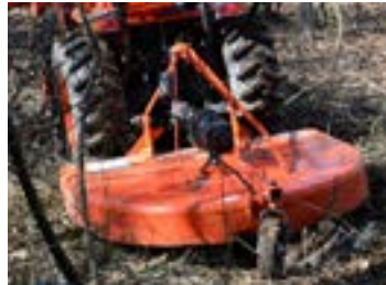
Brush hogs quickly and effectively mow invasive grasses, small shrubs, and small vines.
